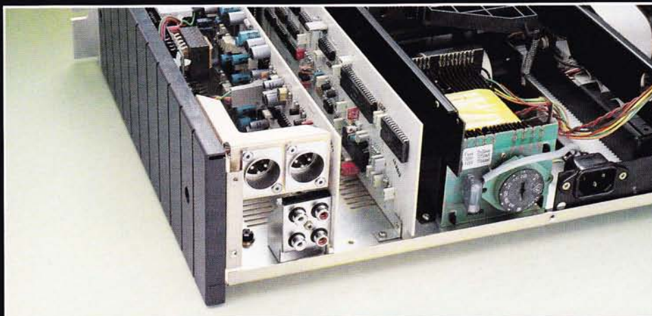
Sockets for audio and control signals: balanced XLR, unbalanced CINCH fixed and variable level, as well as fader start and remote control.
